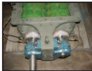
UNIT WITH CINCHSEAL INSTALLED
