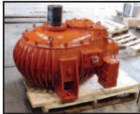
COOLING TOWER UNIT AFTER RECONDITIONING WITH EPOXY COATING
