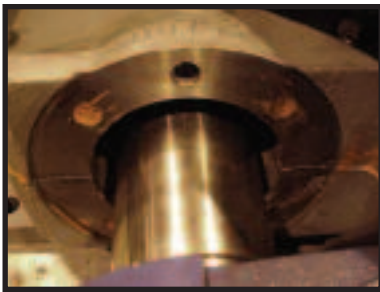
STUFFING BOX HALF FLUSH AFTER MACHINING
